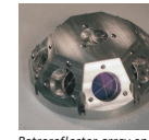
Retroreflector array on Jason, GFO-1, ICEsat, and ADEOS-II ILRS web site photograph
