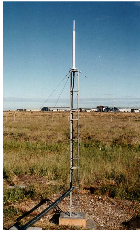
First upgrade (1995): Starec antenna, 3 m tower, good quality guying, mm-level centring and verticality
