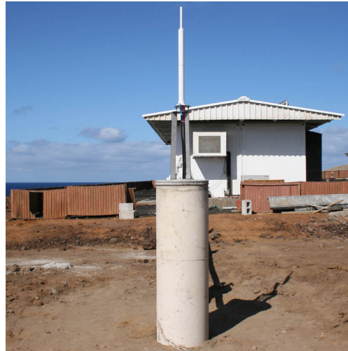
Type II (22%): custom-made tripod on concrete pillar
