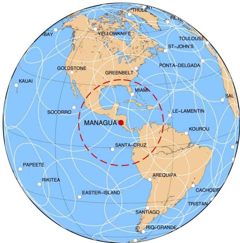
Visibility circle around Managua station for Low Earth Orbit (800km) satellite with 12° cut-off angle over the horizon
