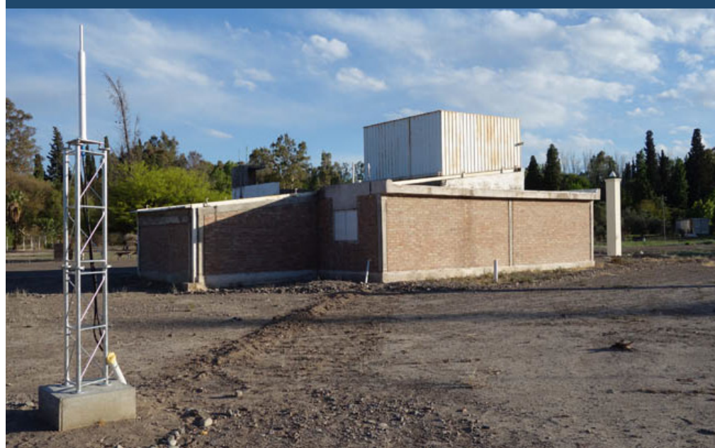
THE DORIS ANTENNA “SJUC” OF SAN JUAN, CO-LOCATED WITH SLR AND GNSS
