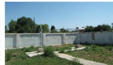
The new DORIS antenna "KIVC" and the new GNSS antenna "KITG"
