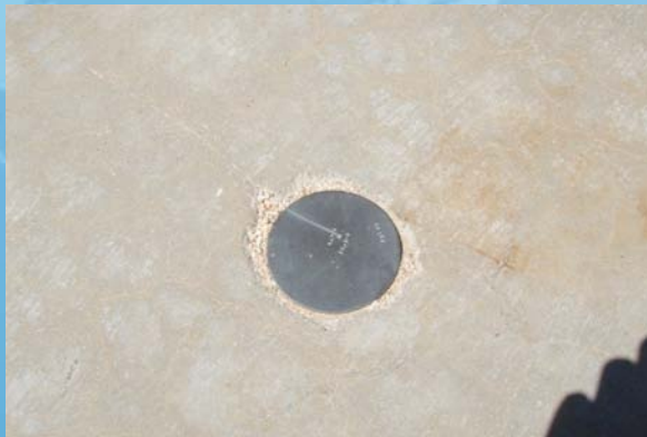
Concrete pad with old mobile VLBI marker (south of old Goldstone DORIS site)
