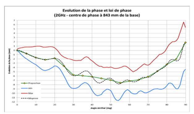
Figure 7: Starec-Cobham TYPE D 2 GHz phase correction
