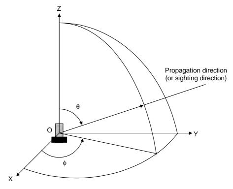
Figure 2: Antennas reference frame (O = phase centre)
