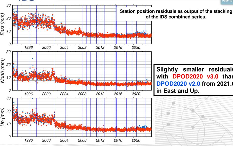
Slightly smaller residuals with DPOD2020 v3.0 than **DPOD2020 v2.0 from 2021.0** in East and Up.
