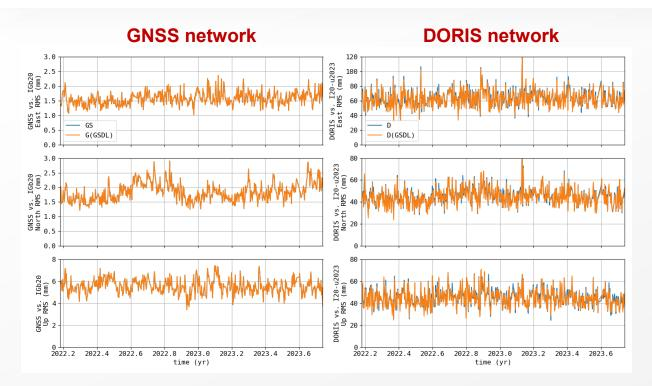
RMS of station positions of GNSS and DORIS solutions are the same in both the individual (GS et D) and combined (GSDL) solutions.
