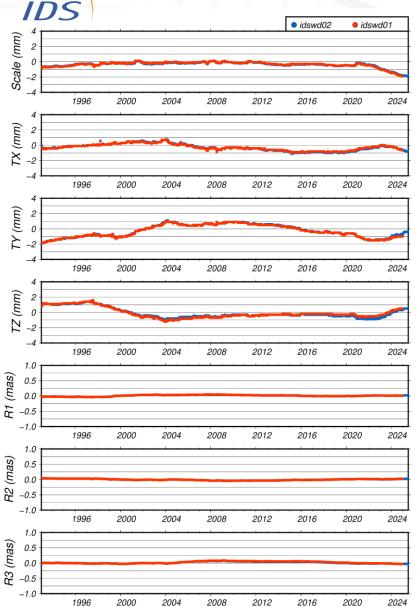
Helmert parameters of the weekly propagations of ids25d01 and ids25d02 wrt ITRF2020-u2023 without annual and semi-annual corrections.
