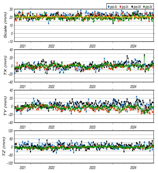
Helmert parameters wrt DPOD2020 v4.0
