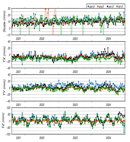
Helmert parameters wrt DPOD2020 v4.0
