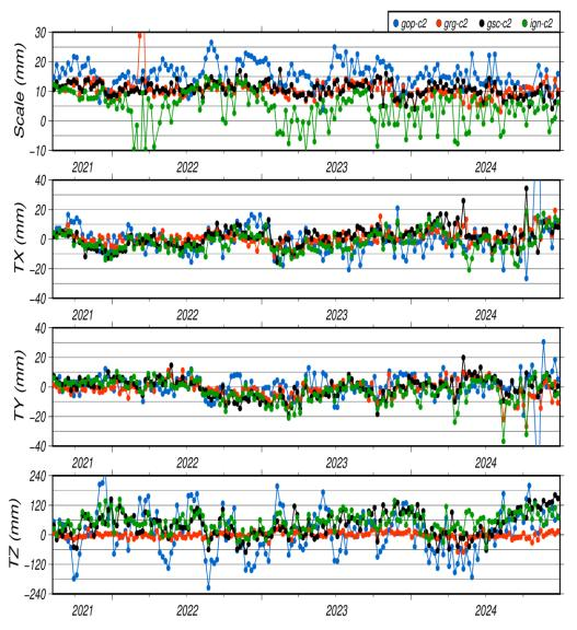
Helmert parameters wrt DPOD2020 v4.0
