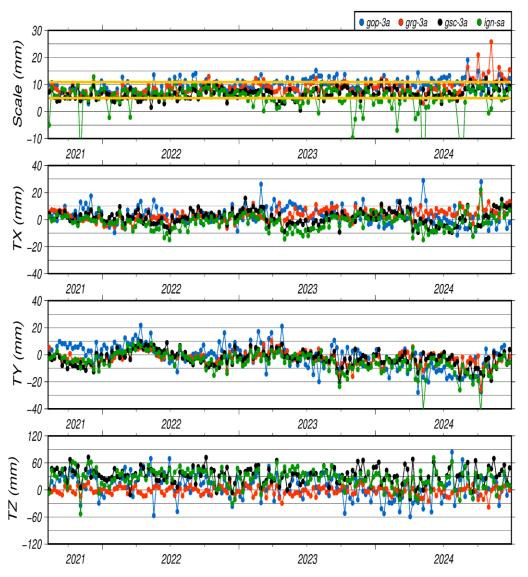
Helmert parameters wrt DPOD2020 v4.0
